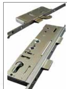
Yale The Mantis 3 Lock can be used with a Lever Lever or Lever Pad handle, the lock consists of ten locking points, four roller cams, two linear bolts, two hooks, a thumb latch and a dead bolt.
